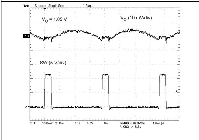
Figure 12. Voltage Ripple at Output ( $I_O = 3\text{ A}$ )
