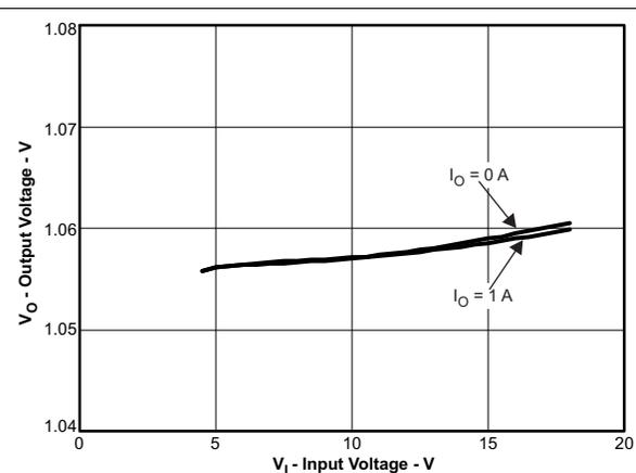
Figure 9. 1.05-V Output Voltage vs Input Voltage
