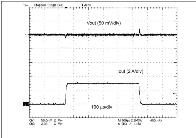
Figure 10. 1.05-V, 0-A to 3-A Load Transient Response
