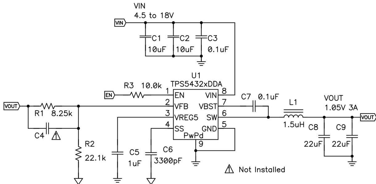
Figure 7. Schematic Diagram
