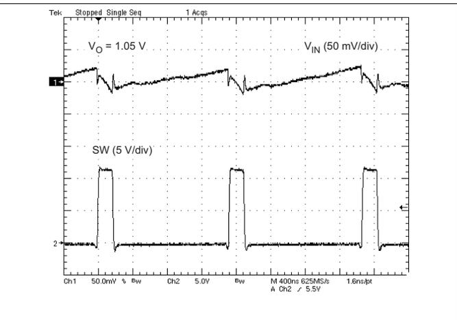
Figure 13. Voltage Ripple at Input ( $I_O = 3\text{ A}$ )
