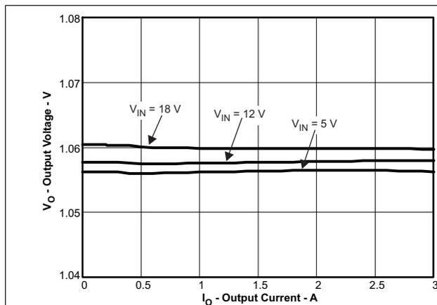
Figure 8. 1.05-V Output Voltage vs Output Current
