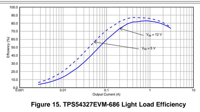
Figure 15. TPS54327EVM-686 Light Load Efficiency
